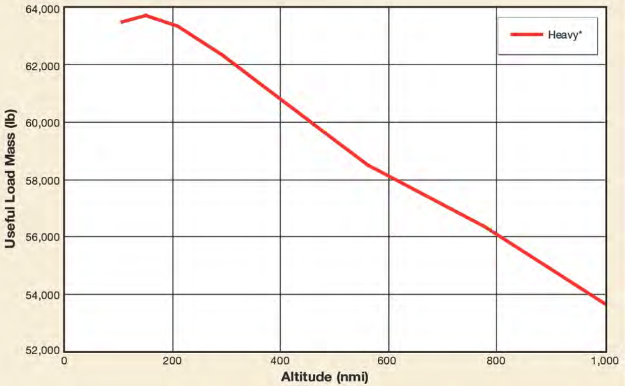
Figure 2-12. Delta IV Heavy LEO Performance Capability, Eastern Range (28.7 deg)
