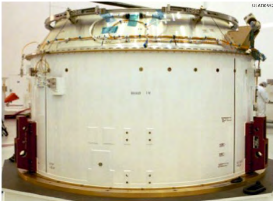
Figure 5-30. ULA Payload Adapter Configuration — PSR with LVA
